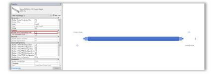
Each component has one end open, and one end with the option to toggle the joint pack on/off (in the instance parameters). This is to enable the production of an accurate Bill of Materials with correct number of joint packs
