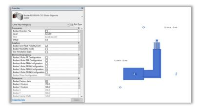
IMPORTANT - Please ensure that all element connectors are placed at the same location when joining to the previous / next piece to create a completed run. We suggest using the Align tool between two external casings of two separate elements.
