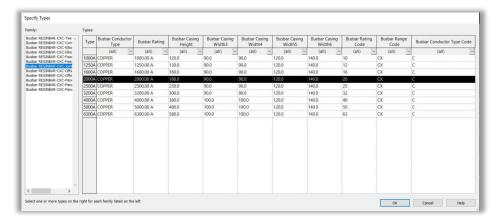
3d. When selecting 'Feeder Straight' lengths in the Insert Table, please select 1m, 2m & 3m lengths from the rating you desire.
